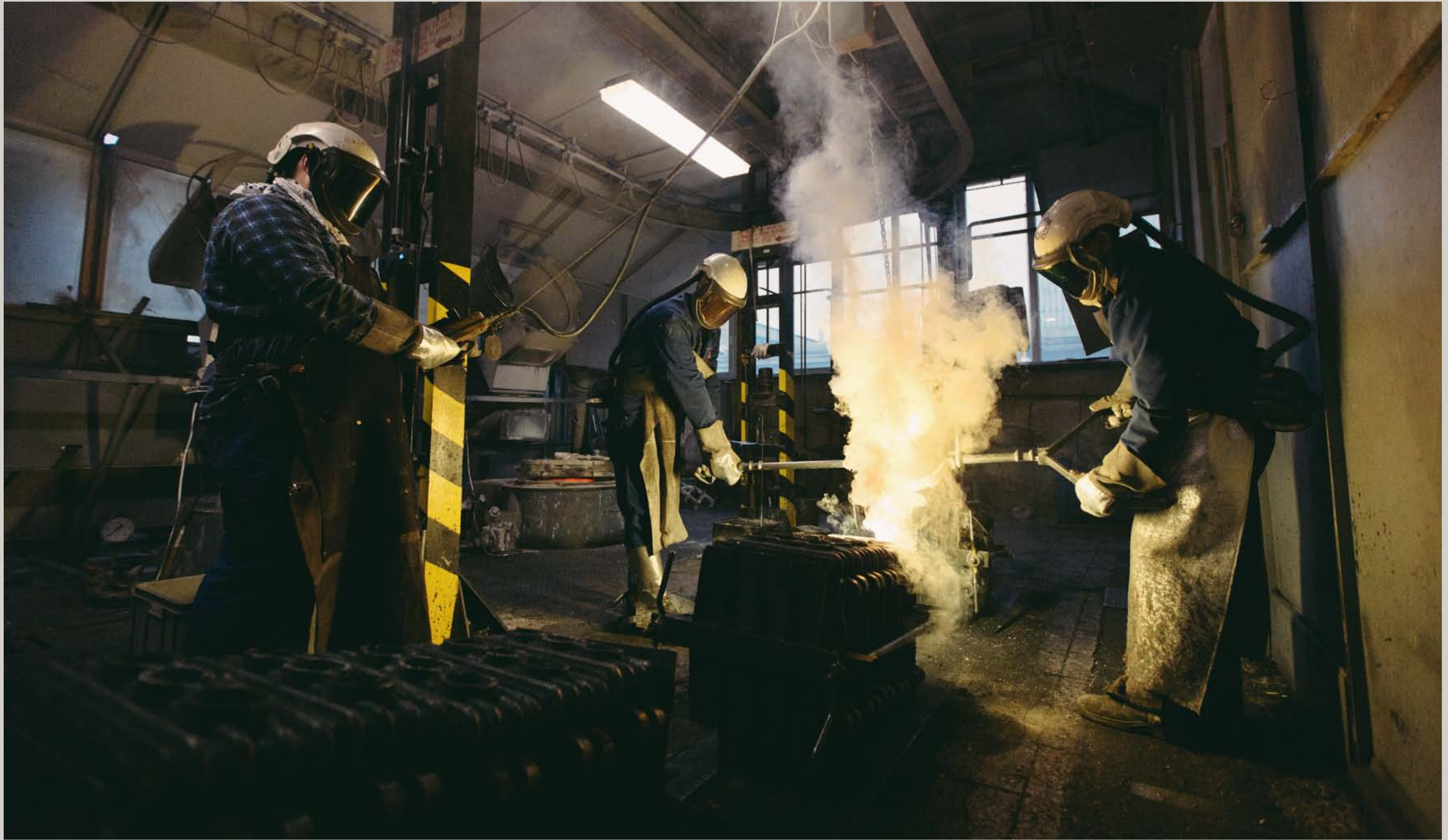
Metal components are created using a traditional process of manual gravity casting. This allows us to achieve the highest quality and precision in detail.
